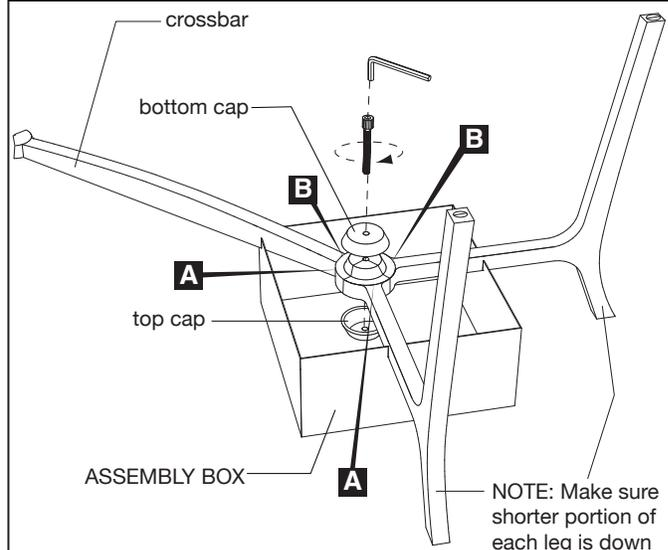
Position **leg A**, **leg B** and **crossbar A/B** into corresponding slots of **assembly box** as shown. Make sure letter labeled on each **leg** corresponds with letters labeled on **crossbar**. Attach **top and bottom caps** onto center of leg/crossbar assembly with 1 **bolt** as shown. Secure bolt with an **allen wrench**. Repeat steps for the other side of **crossbar C/D** with remaining **leg C** and **leg D**.
