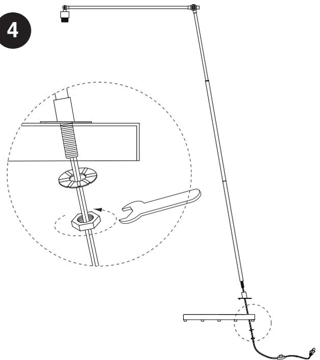
Fit threaded end of *lower upright* into base support and through base as shown. Fasten connection from below with the *lock washer* and *hex nut*, securing the assembly with the **hex wrench**.
