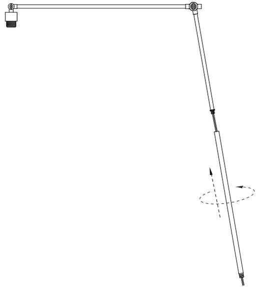
Fit threaded end of *middle upright* into assembly and turn counter-clockwise to secure.
