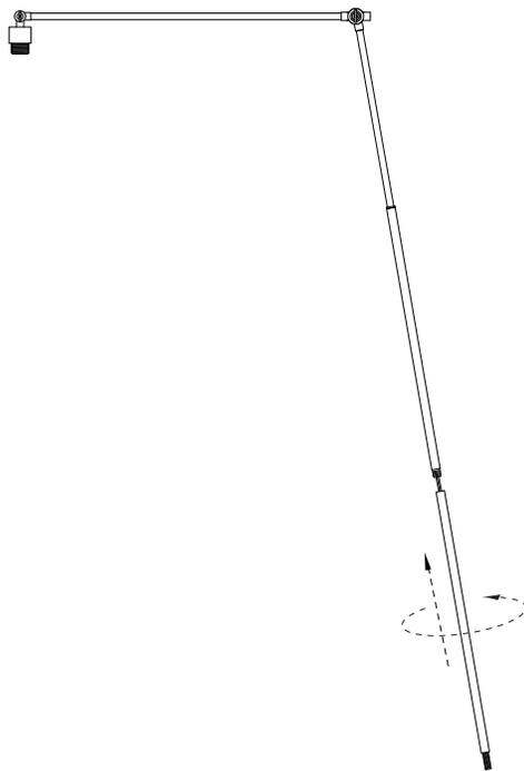
Fit threaded end of *lower upright* into assembly as shown. Turn counter-clockwise to secure.
