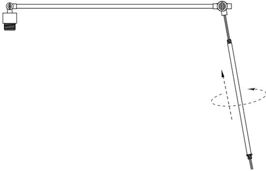
Fit threaded end of *top upright* into assembly as shown. Turn counter-clockwise to secure.
