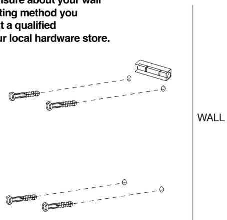
1 Determine the location for the wall sconce. Using a **level**, position **wall sconce assembly** and mark 4 hole positions on the wall. Set wall sconce assembly aside. Drill a pilot hole in the wall stud. If the wall stud is not available, drill a hole in the wall that is slightly smaller in diameter than the anchor. Insert 4 **plastic anchors** into holes. Gently tap **plastic anchors** into the wall until the flange of the anchor is flush.
