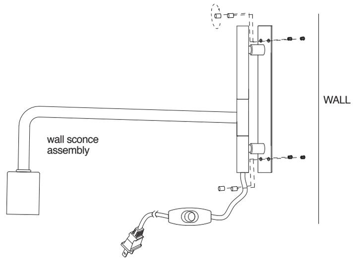
**3** Fit back plate of assembly over studs in wall. Secure studs to assembly with 4 caps.
