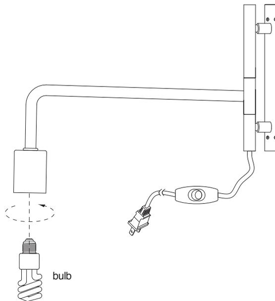
**4** Insert 1- **bulb (included)** into socket. DO NOT EXCEED SPECIFIED WATTAGE. Installation is now complete.
