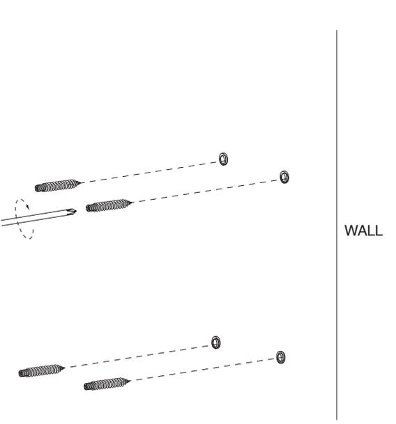
2 Insert 1 **stud** into each **plastic anchor** as shown, and secure using a **phillips head screwdriver**.
