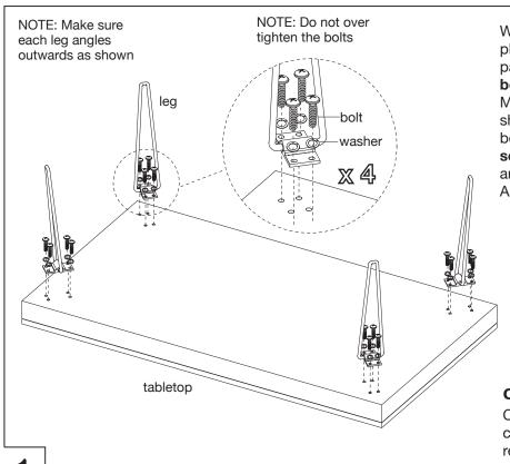
With the assistance of another adult, place **tabletop** upside down on a clean, padded surface. Attach each **leg** with 4 **bolts** and 4 **spring washers** as shown. Make sure each leg angles outwards as shown. Secure, but do not over tighten bolts, with the **phillips head screwdriver**. With the assistance of another adult, position unit upright. Assembly is now complete.
