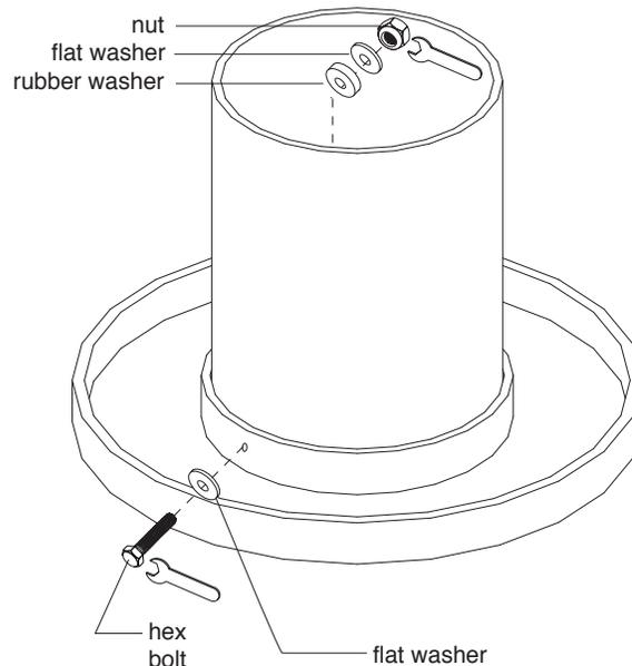
Place **top panel** upside down onto a clean, padded surface as shown. Fit **base** into **top panel** and secure with **2 hex bolts**, **4 flat washers**, **2 rubber washers** and **2 nuts** as shown, with a **hex wrench**. Position table upright. Assembly is now complete.
