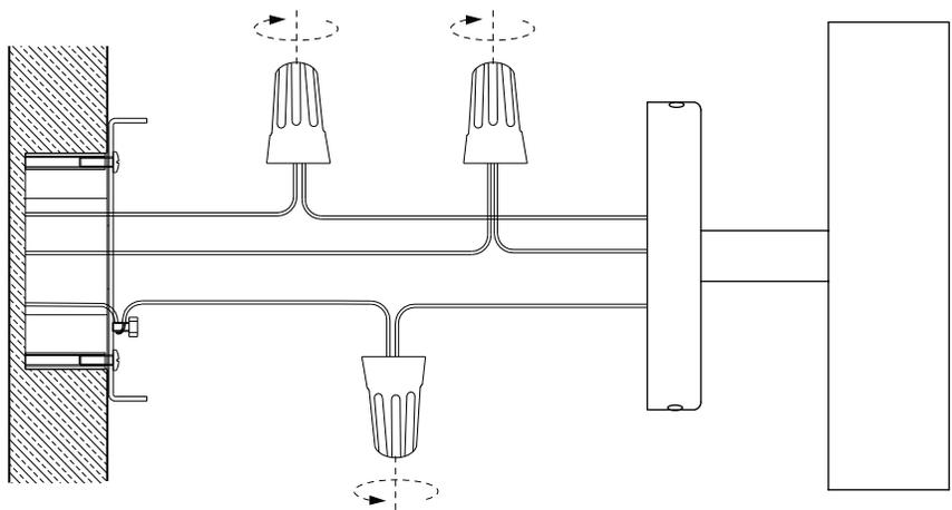
Carefully inspect the fixture wires:
