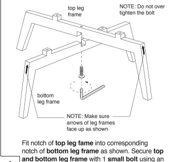
allen wrench. Do not over tighten bolt.
