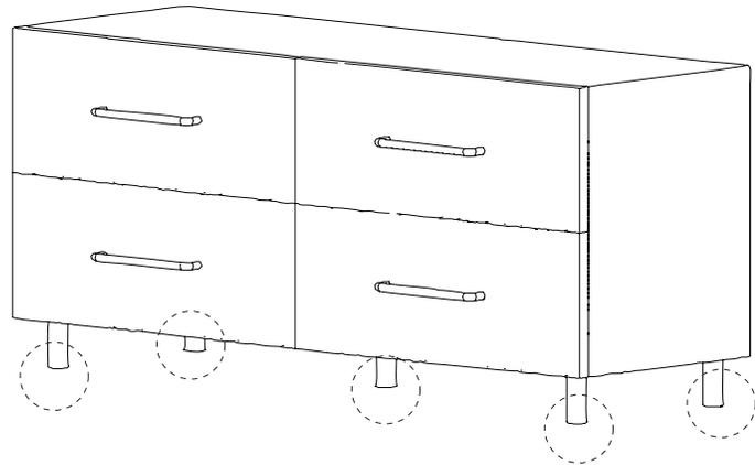
**NOTE:** To increase stability, adjust each leveler until unit is level.
