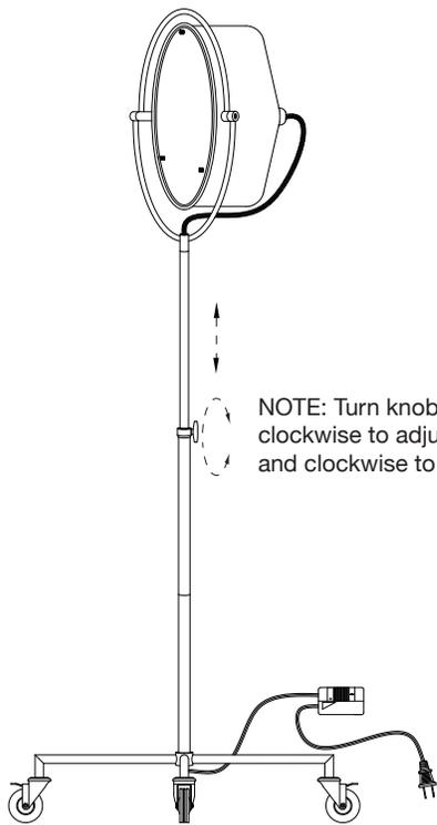
NOTE: Turn knob counter-clockwise to adjust height and clockwise to secure
