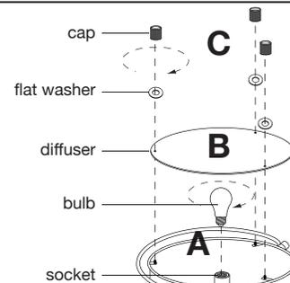
A. Tilt **lampshade** back as shown. Insert 1 - **bulb** (not included) in socket as shown.
